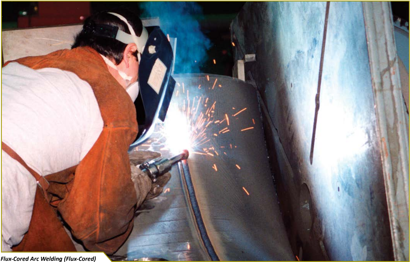
Flux-Cored Arc Welding (Flux-Cored)
