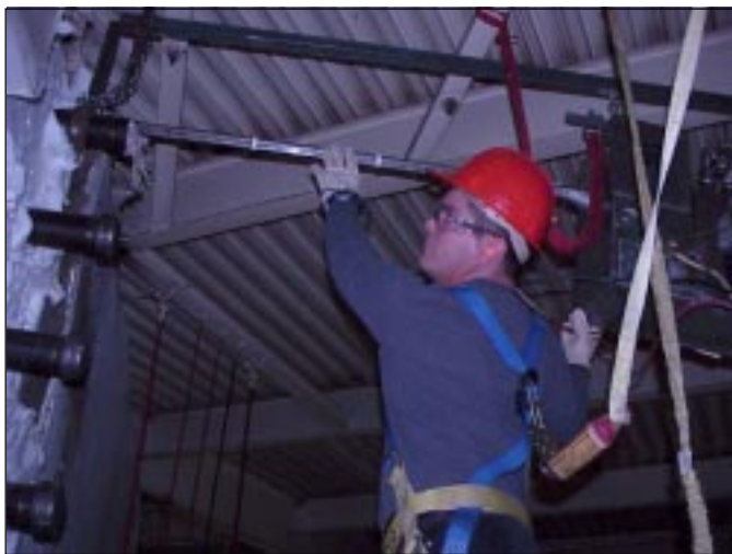
■ The particulate testing probe as it was placed in the stack. The particulate probe tested the amount of particulate coming off the burned biofuel.
